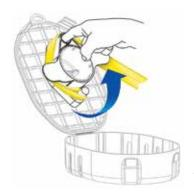
Place loop end over knob and rotate to wind web.
