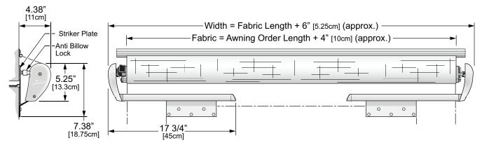
Shown with tall bracket, dimensions are approximate. Actual dimensions may vary based on installation and room configuration.
