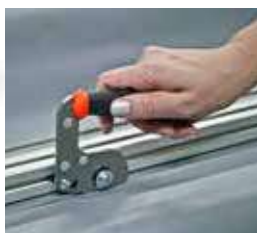
Cut fabric using the rotating cutting blade.
