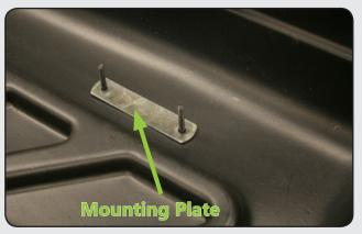
Then slide the mounting plate (C) over the threaded posts inside the cargo carrier.
