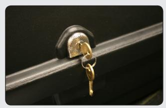
Place key in lock and turn to vertical position as shown. Then remove key. The cargo carrier is now locked. .
