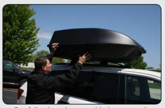
Carefully place the assembled cargo carrier on the top of roof rack cross rails and center on vehicle. Check for clearance of rear hatch and antennas.
