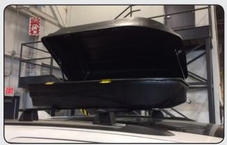
Be sure to place each lid upright in the slotted position to keep from falling during loading and unloading.
