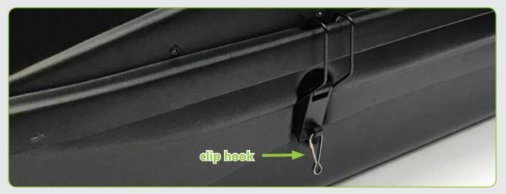
Close cargo carrier. Be sure that BOTH side alignment brackets are NOT visible. Be sure front and back bale latches are in closed position and that the safetly clip hooks are attached.
