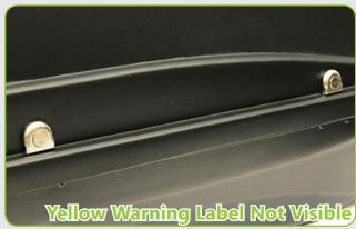
Be sure cargo carrier is fully closed. When this occurs, the yellow warning label will no longer be visible.
