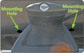
Be sure to align the mounting holes in the box bottom on each side of the cross rails.
