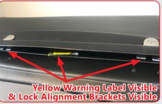
Close up of warning label which should NOT be visible when cargo carrier is properly closed. Be sure both lock alignment brackets are inside the cargo carrier bottom lip to allow for proper lock engagement and a complete seal. **NOTE:** the metal lock alignment brackets should not be visible when the cargo carrier is closed.
