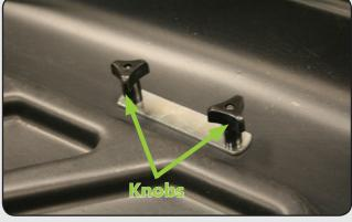
Thread two knobs (B) evenly and loosely – do not tighten all the way at this point. Repeat steps until all 4 mounting brackets (A), all 4 mounting plates (C) are in place and the 8 knobs (B) are loosely in place. Make sure cargo carrier is centered on vehicle. Then tighten all 8 knobs evenly and securely.
