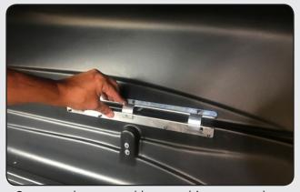
Squeeze the top and bottom hinges together.
