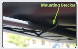
Place the mounting bracket (A) through the pre-drilled holes from below the vehicle cross rails as shown above.
