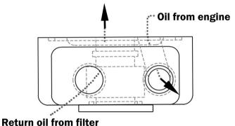
NOTE: A channel is machined 360 degress around the inside of the adapter to allow full flow no mater what position the center nut is.
