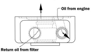
NOTE: A channel is machined 360 degress around the inside of the adapter to allow full flow no mater what position the center nut is.
