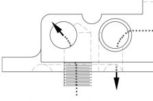
Oil Entry Oil from engine enters adapter and flows to outside of filter
