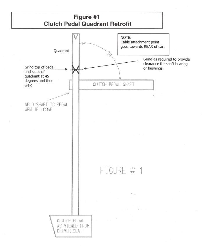
Cable clutches work best with diaphragm type pressure plate. Be sure to install a new release bearing. Adjust cable so it has exactly ZERO PLAY, then adjust one turn tighter on the adjusting nut. This is correct adjustment when using a diaphragm type pressure plate. The release bearing is slightly engaged at all times. This allows for quicker clutch actuation, as well as less clutch pedal travel. This is same adjustment as late model Mustang clutches use. No return spring is required.
