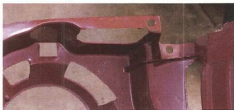
We checked several parts cars at Classic Creations of Central Florida, and they all had broken headlight buckets. Most resemble this one, which is completely separated.
