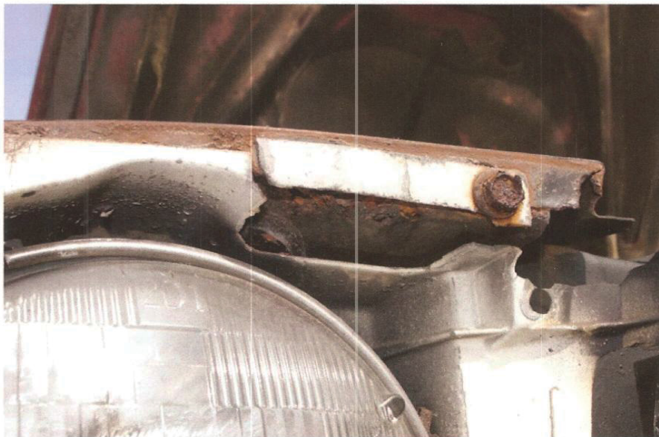
We checked several parts cars at Classic Creations of Central Florida, and they all had broken headlight buckets. Most resemble this one, which is completely separated.
