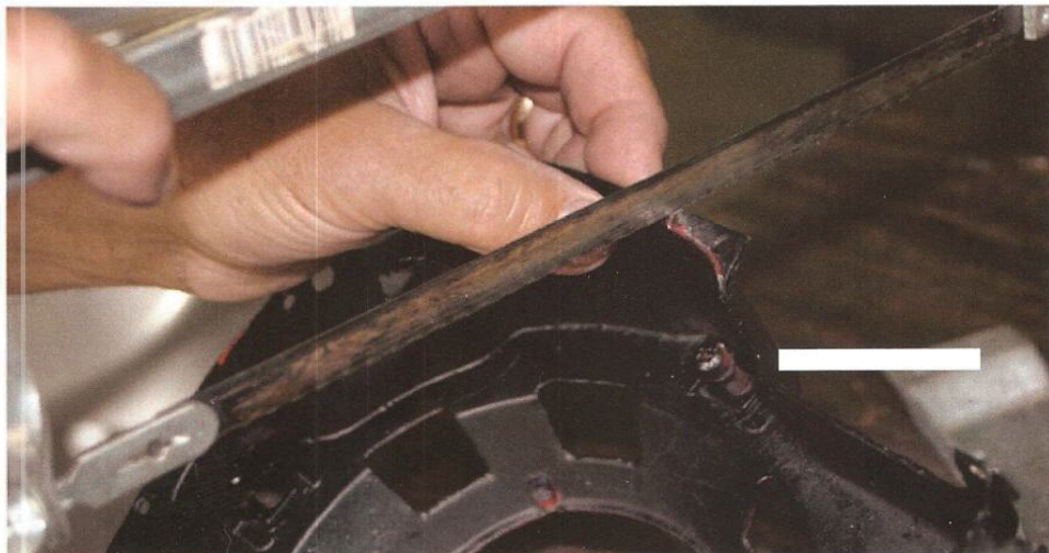
2 There are several ways to remove the remaining section of flange, including the use of a cutting wheel. In some cases, you may be able to break off the cast metal. Merv chose to start the cut with a hacksaw, then used a file to remove metal until he was able to snap off the piece with pliers.
