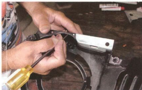
1 After unbolting the bucket from the car and removing the headlight, place the repair patch and note how it's positioned. You'll need to break off or cut the remaining section of the old flange. Here, Merv Rego marks the area that needs to be removed for our bucket repair.
