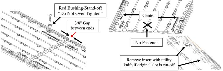
**NOTE:** The screws supplied with this kit are not meant to be used in steel or aluminum, but can be if an 11/64" drill bit is used first to drill a pilot hole. Caution should be used in areas where marker lights and wires have been installed under the trailer deck when installing all fastener.
