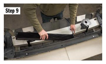
Take the LED from the packing and remove the film from the LED. Then slide in between the plastic and aluminum. It is a tight fit.
