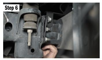
Remove the 8ea (4 on each side) nuts that hold the bumper in place using a 14mm ratcheting wrench.
