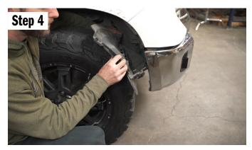
Twist and remove the inner trim from the truck.
