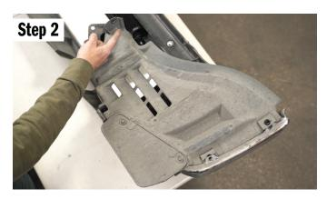
Remove the plastic clip with a pick or screwdriver.
