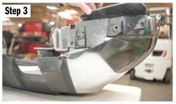
Remove the last 2ea 10mm on the bottom and only the 12mm near the outside of the bumper.
