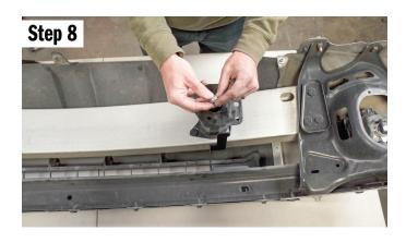
Take a 3/8 bolt and install a washer. then from the top, place the bolt through the mount and then bumper. Then install a washer and lock nut from the bottom. Leave these loose. The washer on the top can fall into the bumper slot, once everything is in place we can adjust this and get it in place.
