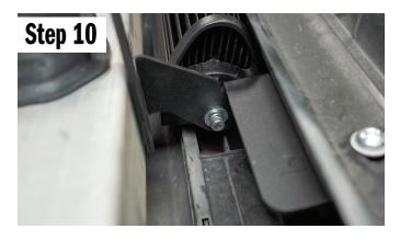
Next we will install the bolts to hold the LED in place. Put a lock washer on the 6mm bolt, then flat washer. Snake your hand in place and put the bolt in the LED. This can be a little difficult. Once both are in, tighten the LED to the mount.
