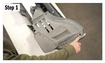
Remove the two outside bolts with a 10mm. Leave the two in the mud flap
