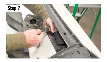
Manuver the bracket in place so that the top tab lines up with the factory slot, and the bottom of the bracket lines up with the frame mount.
