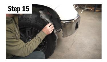
Put the plastic clip, 10mm bolts and 12mm bolts back in place just like you removed, then tighten everything down.
