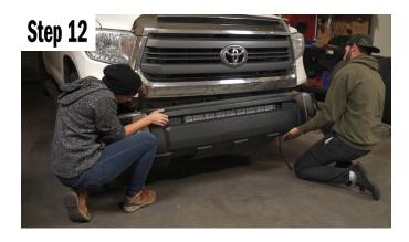
With the LED centered and tightened in place, reinstall the bumper and pay attention that the LED mount slides over the bumper stud as well. Re-install all 8ea nuts and tighten the bumper in place.
