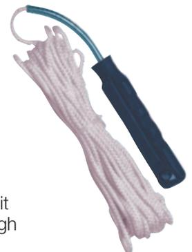
Use our Rope Insert Tool to insert the rope into the groove of rubber backlite gaskets to make the job easier than ever. The contour-grip plastic handle feeds rope through its stem as you pull it around the gasket, and has enough sturdy rope to fit around even the largest backlites or rear truck sliders. Minimum order is one each.
