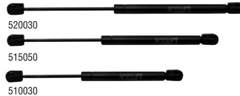
Lift Prop for radius, mitred or fiberglass doors, egress windows, side access windows, or any installation where prop pressure would assist in an opening application. Gas Filled Props have 16 mm diameter black painted steel barrels, 6 mm diameter stainless steel rods, and 10 mm ball socket ends.
