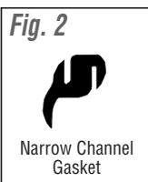
Some pickups are equipped with a wide channel gasket (Fig. 1), on original equipment sliders. These are not acceptable for installation of CRL Truck Sliders, and must be replaced with a narrow channel gasket, such as those shown in (Fig. 2).
