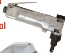
Get a bigger bite and better angle cuts with CRL's Heavy-Duty Air Nibbler. Instead of shearing or sawing, this tool actually "nibbles" aluminum, cold rolled steel, plastics, and an assortment of other metals up to 18 gauge thickness. It will not distort the edges of material being cut, and is designed so you can start cuts in the center of a panel and hold a tight 1/4" radius with great accuracy. 90 P.S.I. required.
