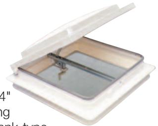
This Van Vent fits in a 14" x 14" hole, and is hinged on the leading edge to allow air circulation. Crank-type operator lifts white plastic lid from closed to a 45° position. Built-in screening keeps insects out. Interior and exterior trim rings are a cream color that can be painted to match the vehicle.
