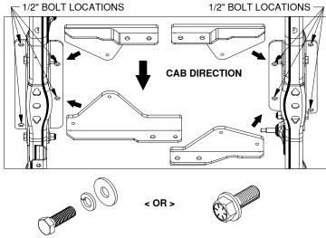
Figure B4: Bottom of truck frame looking up from the back of truck towards the cab
