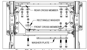
Figure B5: Bottom of truck frame looking up from the back of truck towards the cab
