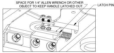
Figure E2: View looking up at latch mechanism of center section.
