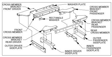
Figure B1: Sideplates and Mounting Kit Exploded View
