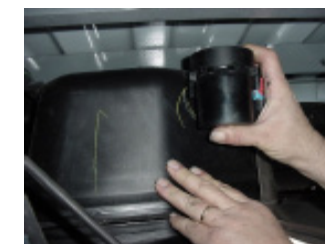
Step 3: Slide fuel valve from bracket.
