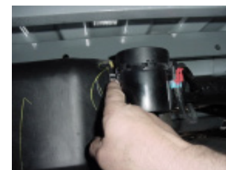
Step 2: Disengage the locking pin.
