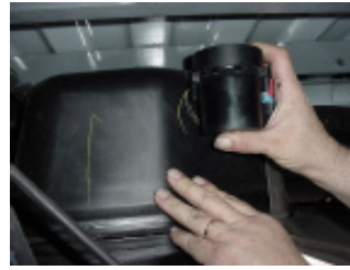
Step 3: Slide fuel valve from bracket.
