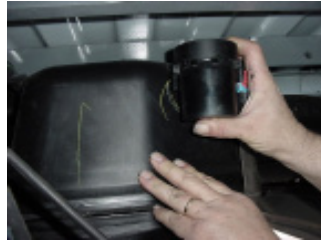
Step 3: Slide fuel valve from bracket.
