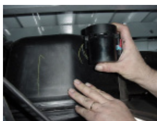
Step 3: Slide fuel valve from bracket.
