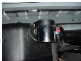
Step 1: Locate the fuel valve.
