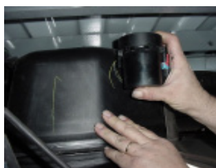
Step 3: Slide fuel valve from bracket.
