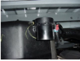
Step 1: Locate the fuel valve.
