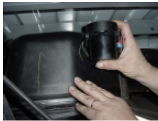
Step 3: Slide fuel valve from bracket.
