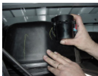
Step 3: Slide fuel valve from bracket.
