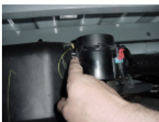
Step 2: Disengage the locking pin.
