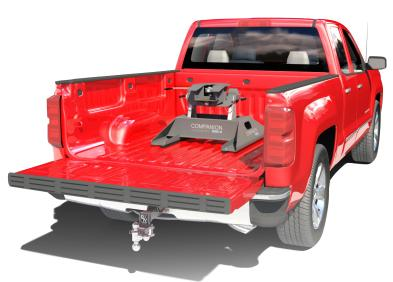
manufacturers calculate how much a truck can safely accelerate and stop before assigning a tow rating. For Gross Weight Ratings, the truck's tires, frame, and suspension must be able to bear the load. It's important to never exceed the ratings assigned by the truck, trailer, or hitch manufacturers for the specific equipment you are using.
