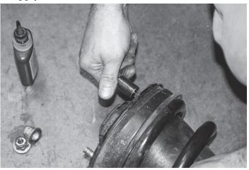
8. Install the lift spacer.
