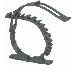
**4.** The strap is divided into three sections. The first holds objects up to 3", the second 5" and the third up to 7". If desirable, excess sections can be trimmed of with wire cutters or scissors.
