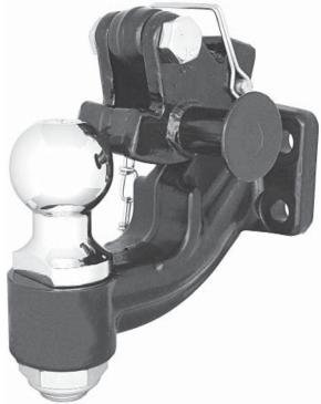
**4.** To close latch, pull plunger, rotate latch closed and release plunger. Plunger must be fully engaged to lock the latch. Assembly safety pin.
