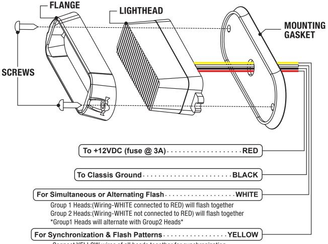
Connect YELLOW wires of all heads together for synchronization \*All heads must be set at the same pattern attention: Lightheads will not sync on the random pattern (pattern 1)
