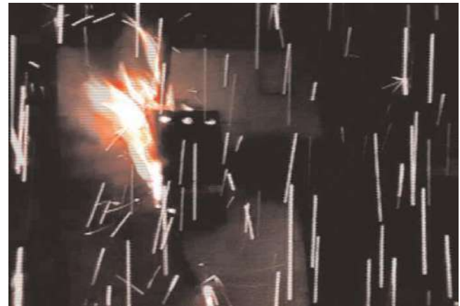
Photo (later in sequence) of 3-pole device during test of individual single-pole interruption of a fault current beyond the tested values specified by the UL standard
