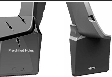
Identify which of the enclosed fasteners best suits your Fender Flare and Mud Flap combination. Hold the Mud Flap up to your Bushwacker<sup>®</sup> Fender Flare and mark the hole locations using a grease pencil. Pre-drill holes in the Fender Flare where you will use plastic push fasteners. Pre-drilled holes are not necessary if using screws.
