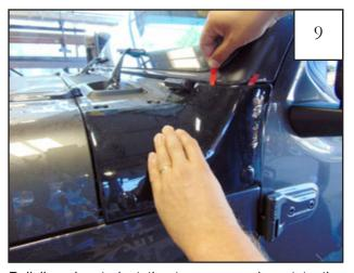
Pull liner located at the top corner closest to the center of the windshield. Press down on entire length of part applying strong pressure to the taped areas.
