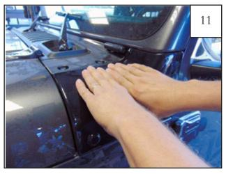
Apply strong pressure for 30 seconds on each section of the part to ensure proper adhesion. *NOTE:* The tape reaches maximum adhesive bond after 24 hours of contact.
