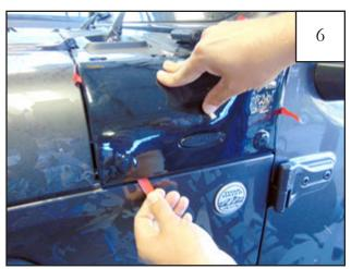
Pull liner of lower tape strip. Press down on entire length of part applying strong pressure to the taped areas.
