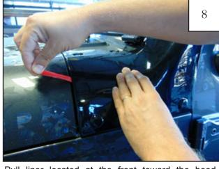
Pull liner located at the front toward the hood. Press down on entire length of part applying strong pressure to the taped areas.
