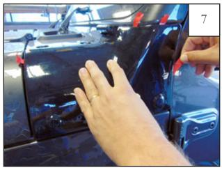
Pull liner located at the rear toward the door. Press down on entire length of part applying strong pressure to the taped areas.
