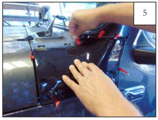
Begin by pulling the top tape liner first. Press down on entire length of part applying strong pressure to the taped areas.
