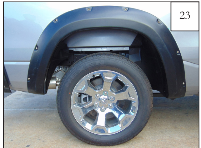
Completed rear flare installation.
