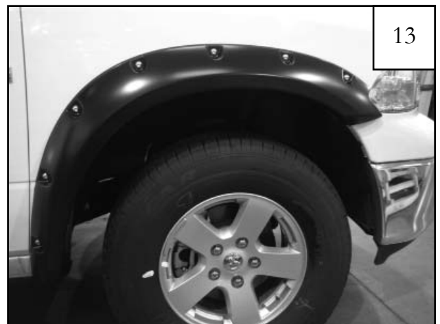
Completed front flare installation.
