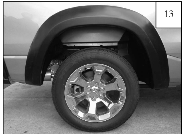
Completed rear flare installation.
