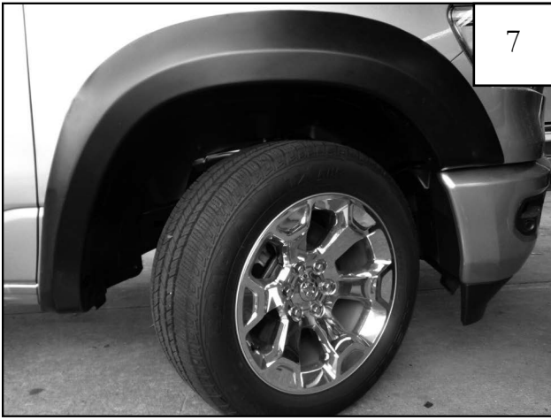
Completed front flare installation.
