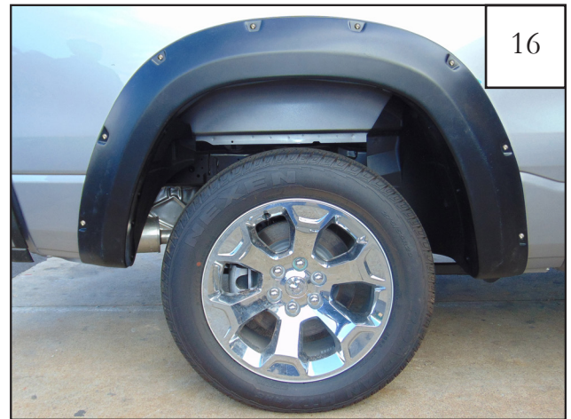
Completed rear flare installation.
