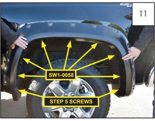
Install rear flare using (7) SW1-0058 truss screws and the (2) outboard screws removed in Step 5.
