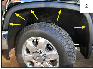
Remove (5) factory installed screws.
