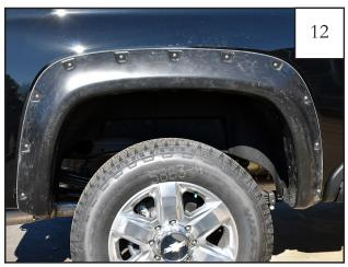
Fully tighten all fasteners, then replace the rear wheel as instructed in your user's manual. Rear flare installation is complete. Repeat procedure for opposite side.
