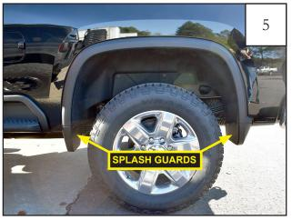
Remove the rear wheel as instructed in your user's manual. Remove the rear splash guards using a T-15 Torx driver. Retain screws for later use.
