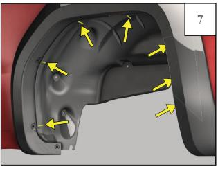
While holding the rear flare in place, mark the flare's (7) hole locations using a grease pencil. Remove flare after marking.
