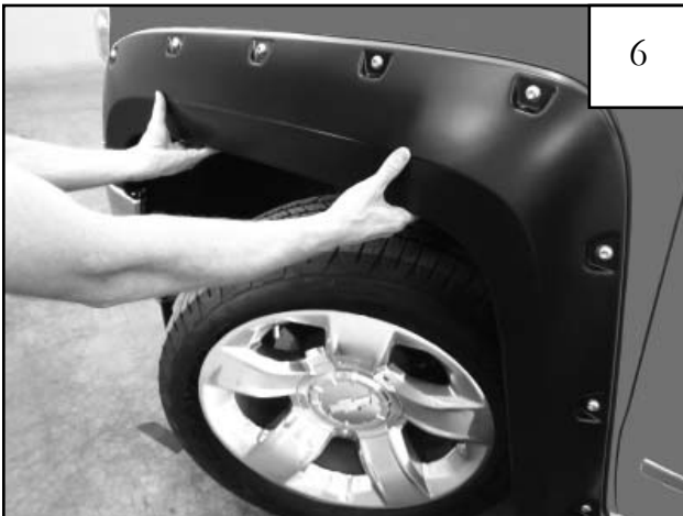
To mount the flare into position, hold the flare 2-3" inches below the top lip of the wheel well. Push in and slide up to allow flare to fully seat against the wheel well opening.
