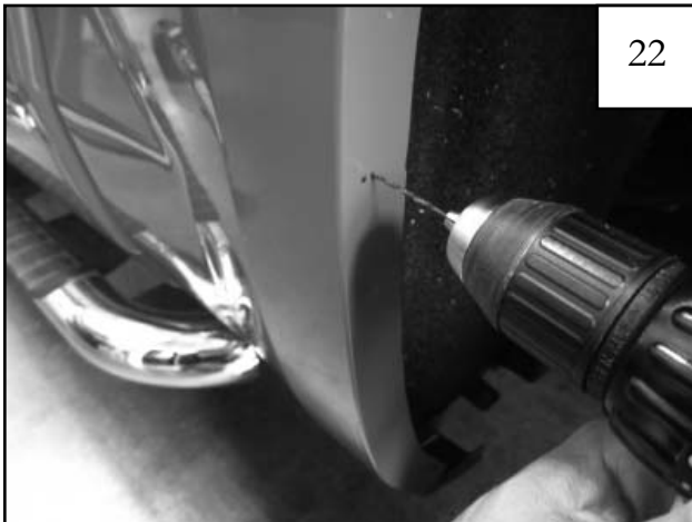
Using a 3/32" drill bit, drill pilot holes at the marks made in Step 21.
