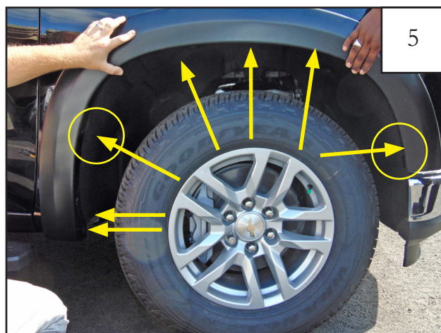
Hold flare to vehicle and note the approximate hole locations in the flare.
