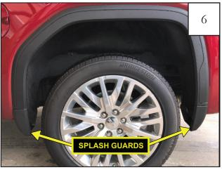
Remove the rear wheel as instructed in your user's manual. Remove the rear splash guards using a T-15 Torx driver. Retain screws for later use.
