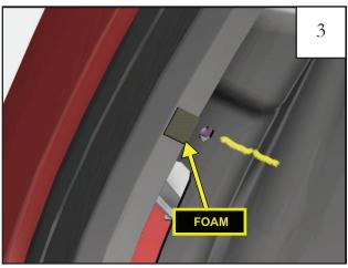
Install (6) MT1-0034 foam tabs around the stock fender trim where the grease pencil marks were made.
