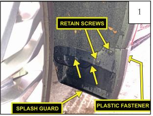
Remove the front splash guard using a T-15 Torx driver and retain (2) screws for later use.
