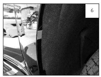
Install supplied Tab (MT1-0034) at each location marked in Step 5.
