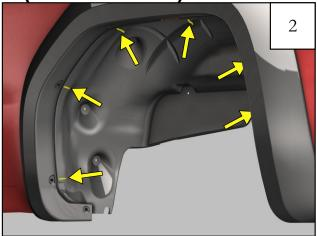
While holding the rear flare in place, mark the flare's (6) hole locations using a grease pencil. (Wheel only removed for visual clarity.)
