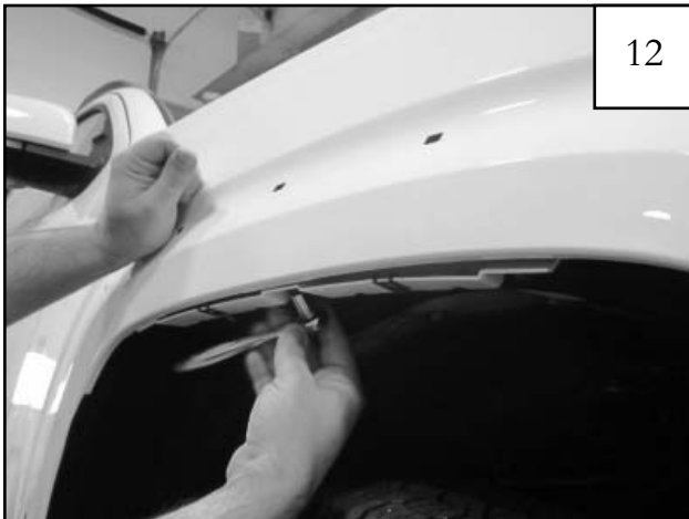
Using three supplied screws (SW1-0036), attach bracket to wheel well. Tighten all screws.
