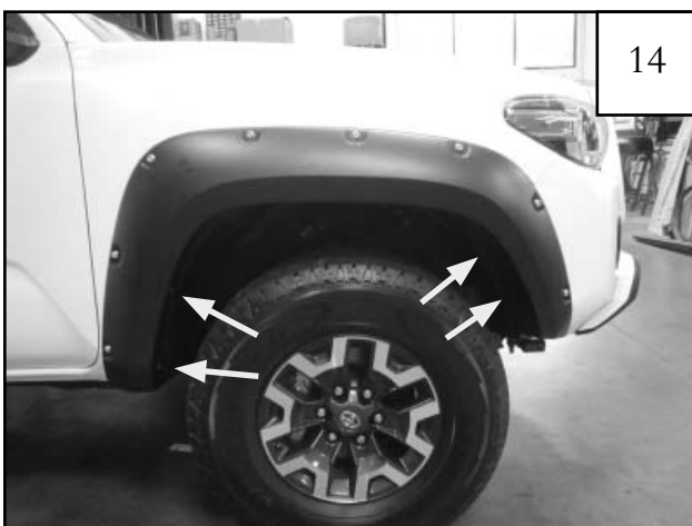
Still holding flare to fender, install supplied screws (SW1-0036) into remaining mounting holes (4 places).
