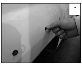
Using a clockwise twisting motion, remove eight factory plastic clips from fender. See step 9.
