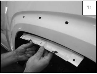
Line up the holes in the inner piece with the three uppermost factory holes. NOTE: Driver's side inner piece is marked with an "LF" and passenger's side inner piece is marked with an "RF"
