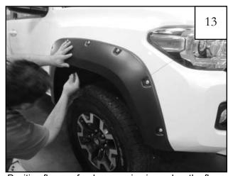
Position flare on fender, pressing inward on the flare, line up the flare mounting holes with the mounting clips on the bracket. Install 2 supplied screws (SW1-0036) through the flare and into the clips on the bracket. Do not tighten.
