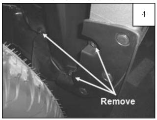
If factory mud flap is installed, remove three factory screws from the mud flap. Save screws for reinstallation.
