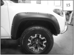
Tighten all screws. Installation Complete.
