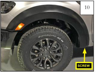
Reinstall (1) T-25 Torx screw previously removed from rear of the flare in Step 2.
