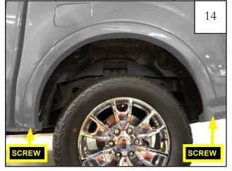
Remove (2) factory installed screws from under the fender trim using a T-25 Torx driver. The screws will be re-used to install the rear flare.
