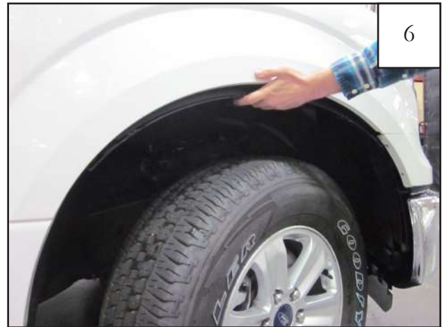
Line up the holes in the inner piece with the three uppermost factory holes. NOTE: Driver's side inner piece is marked with an "LR" and passenger's side inner piece is marked with an "RR".
