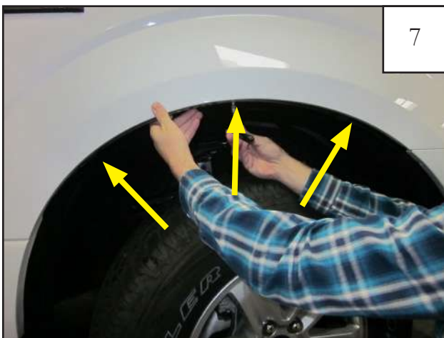
Using a 7/32" socket wrench, reinstall the factory screws through the inner piece.
