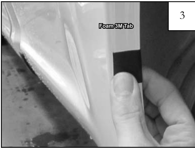
Wrap a Foam Tab (MT1-0034) around the wheel well sheet metal, centered over the mark made in Step 2.
