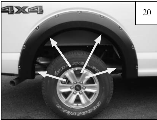
20 While holding flare to vehicle, start supplied screws (SW1-0058) through the four topmost mounting holes in flare and into the clips installed in Step 18.
