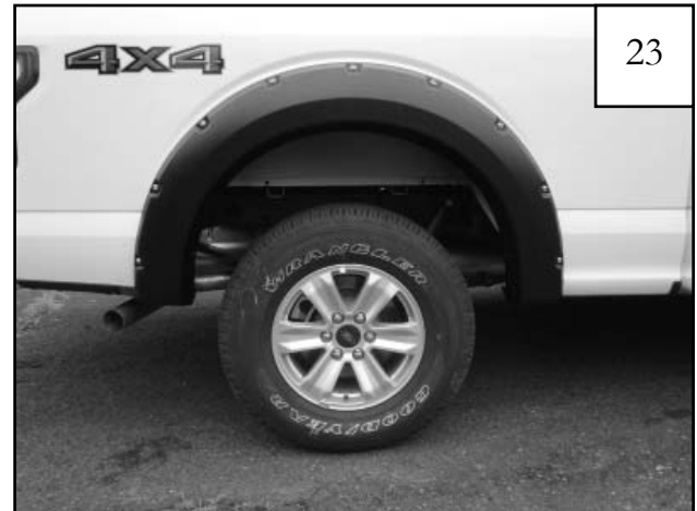
23 Completed rear flare installation.
