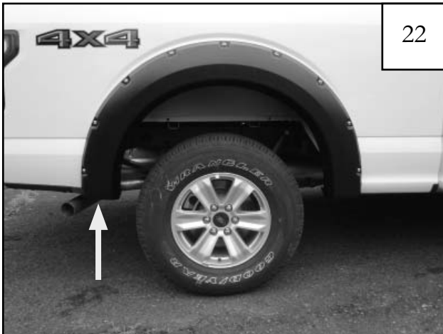
22 Install supplied push retainer (RV1-P0006) into flare and through factory hole at rear of wheel well.
