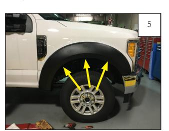
Position flare on fender, pressing inward on the flare, line up the flare mounting holes with the mounting clips on the inner piece. Install 3 Phillips Truss Screws (SW1-0058) through the flare and into the clips on the inner piece. Do not tighten. (3 locations)
