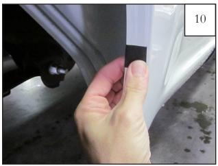
Wrap a Foam Tab (MT1-0034) around the wheel well sheet metal, centered over each of the upper four marks made in Step 9. Place a Mylar Tab (MT1-0014) at the mark made on the lower front of the wheel well.
