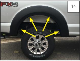
While holding flare to vehicle, start supplied screws (SW1-0058) through the four topmost mounting holes in flare and into the clips installed in Step 12.
