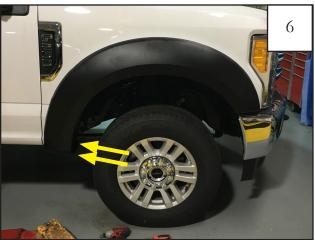
Still holding flare to fender, re-install remaining factory screws removed in Step 1 using 7mm socket and wrench. Tighten all screws.
