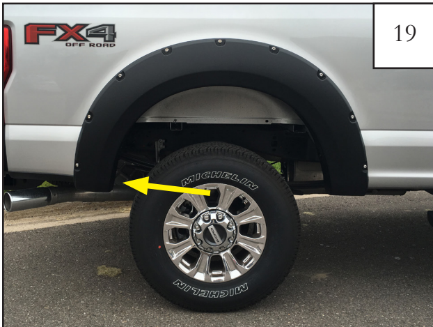
19 Install supplied push retainer (RV1-P0001) into flare and through factory hole at rear of wheel well.
