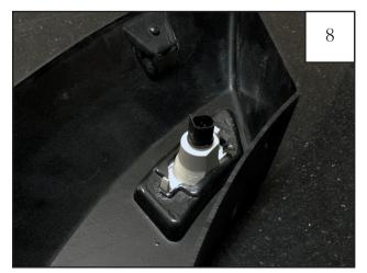
Install the turn signal assembly into the front driver side flare.
