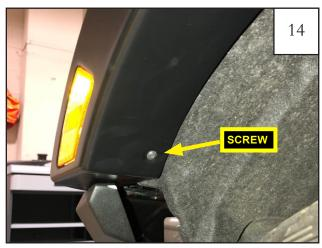
Install (1) truss screw (SW1-0050) through the front hole in the flare into the "S" spring clip using a #2 phillips screwdriver.
