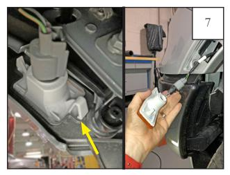
Squeeze the lower tab on the back of the turn signal assembly and remove from the truck. Carefully turn the wiring harness counter-clockwise and separate the bulb/wiring harness from the turn signal assembly.
