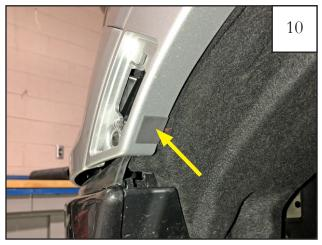
Install (1) black mylar tab (MT1-0014) around the edge of the fender trim aligned with the grease pencil marking.
