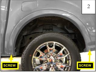
Remove (2) factory installed screws from under the fender trim using a T-25 Torx driver.
