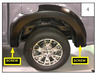
Reinstall (2) T-25 Torx screws previously removed from rear flare in Step 2.
